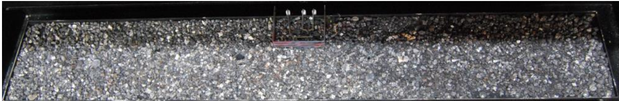
Photo 6 – Vermiculite spread on burner
