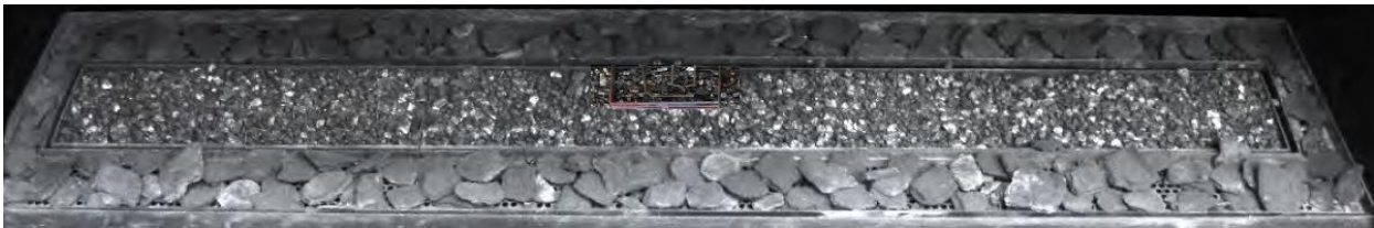
Photo 7 – Vermiculite Chips spread around burner
